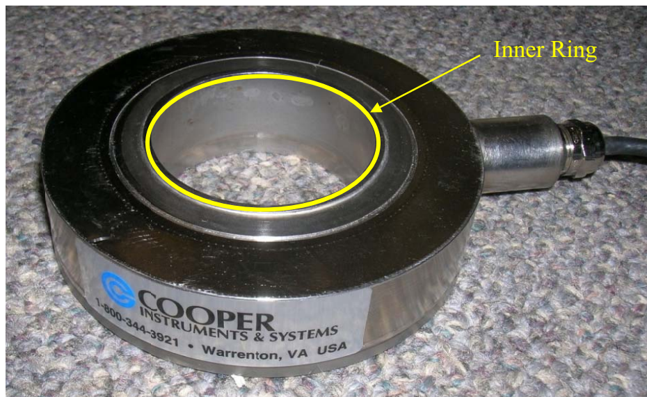
Figure 85 - Load Cell Loading Surface: Inner Ring
