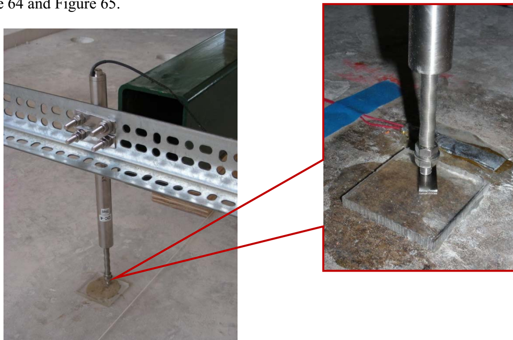
Figure 57- Differential Transducers (DCVTs)
