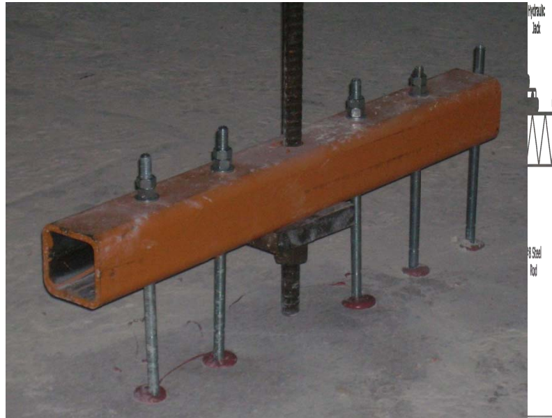
Figure 48 – Anchoring System using Hilti Rods: Ground Level
