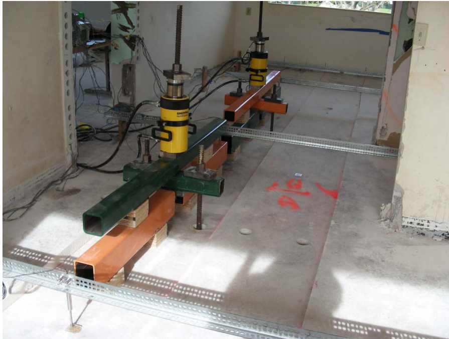
Figure 52 – Loading Setup (Hydraulic Jacks)
